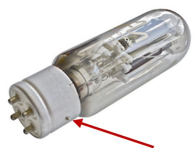
Inspect a VT-4C valve and you will notice that there is a small 'pin' protruding from one side of the valve base; this locating pin ensures that the valve can only be correctly inserted into the amplifier in one way.
