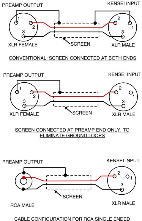
PREAMP OUTPUT TO XLR BALANCED AMPLIFIER INPUT
